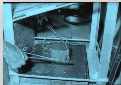
1987 - Preparation of Iridium-192 wires for manual after -loading
